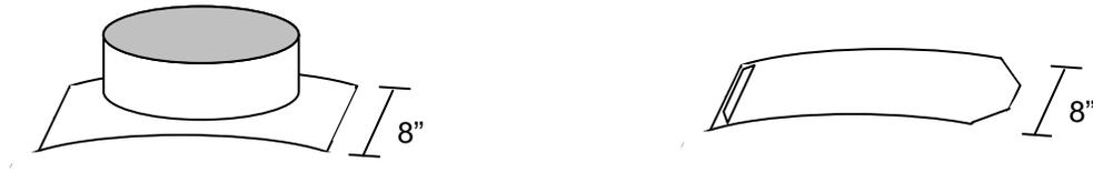
Figure 3. Flange for attaching exhaust stovepipes to kiln C-brackets (left) and damper plate (right).
