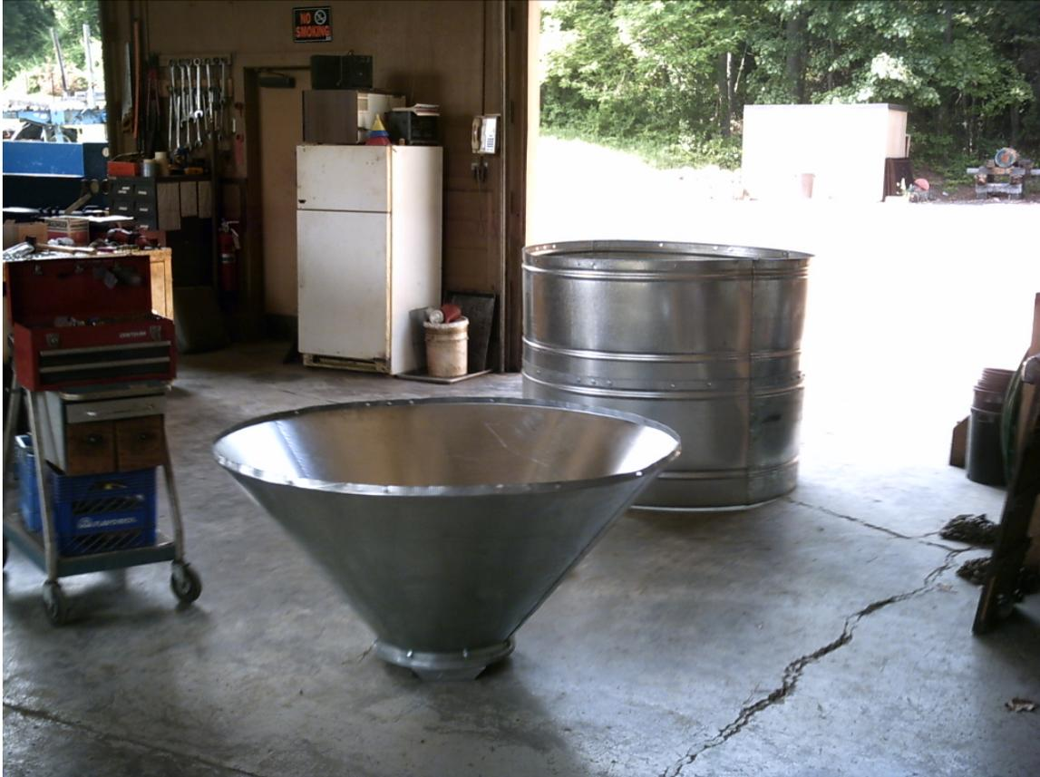
Figure 4. Kiln body and bonnet unmodified from pre-fabricated bulk bin kit.
