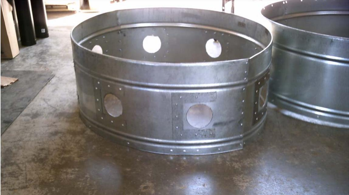
Figure 5. Lower body section with cutout holes and C-brackets installed.
